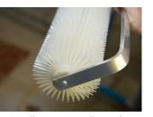
Porcupine rollers are an excellent tool to use in between bucket pours to break the surface tension of the product.
