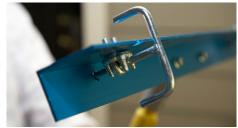
Gauge rakes are used to measure the product depth and help spread the material quickly.
